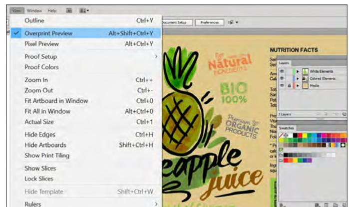
Turn on "Overprint Preview" gives an accurate view of the file's setup within the application before exporting and printing ("SpotColor\_White" swatch is set to green in this example)
